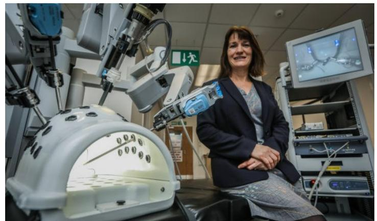
**The four thin arms are inserted into a patient through strategically placed incisions < 2 cm long. These are manipulated by surgeons using hand and foot controls enabling them to operate without the need for large incisions, facilitating greater precision and faster recuperation.**
